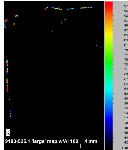
Sr was observed in the sample spectrum, but backscatter is contributing to artificial signal on map.
