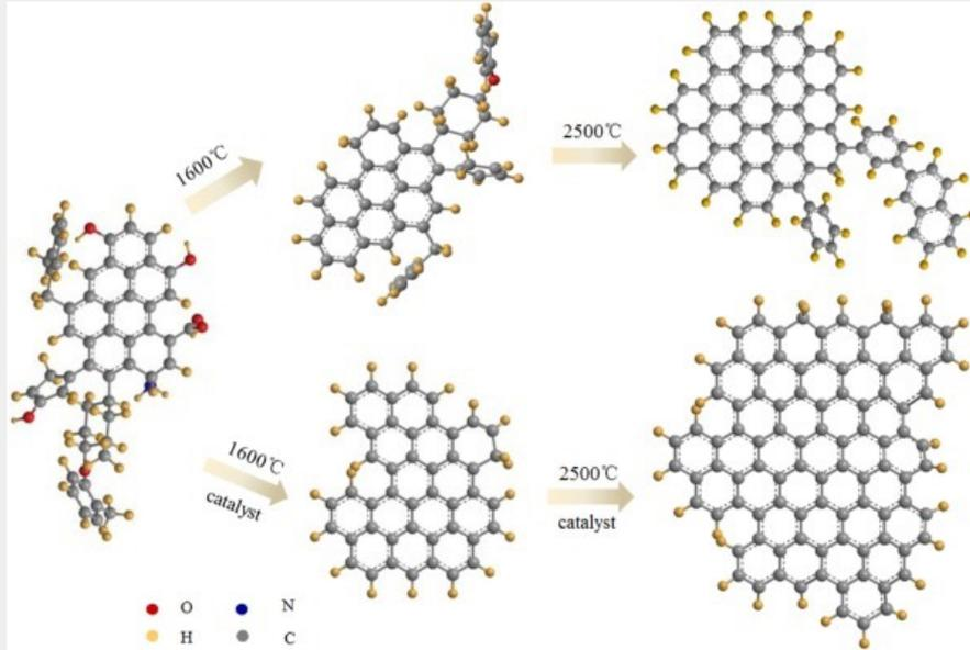
Simple graphitization of coal is possible by high temperature treatment above 2800 C
