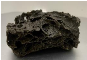
CHAR INSULATION FOAM (CIF)
