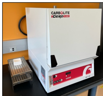
Carbolite Gero Ashing Furnace in the GTL at the University of Wyoming's School of Energy Resources.
