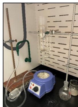
Soxhlet Solvent Extractor in the GTL at the University of Wyoming's School of Energy Resources.
