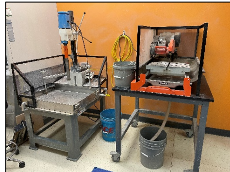
Diamond Core Drilling & Cutting System in the GTL at the University of Wyoming's School of Energy Resources.
