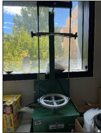
Motorized Sieve Shaker in the GTL at the University of Wyoming's School of Energy Resources.
