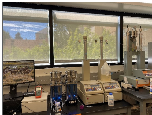
Teledyne ISCO 260D Syringe Pumps in the GTL at the University of Wyoming's School of Energy Resources.
