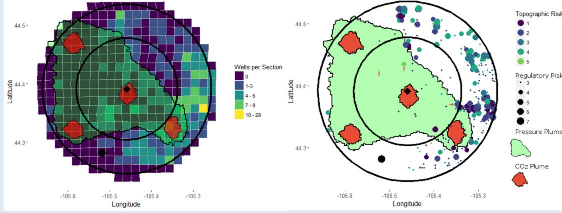
Figure 3. Risk as shown in Figure 1 and 2 from wells penetrating the Opeche confining layer and the CO<sub>2</sub>/pressure plume extent of a simulation storing 50 million tonnes of CO<sub>2</sub> in the Minnelusa formation, underlying the Opeche.
