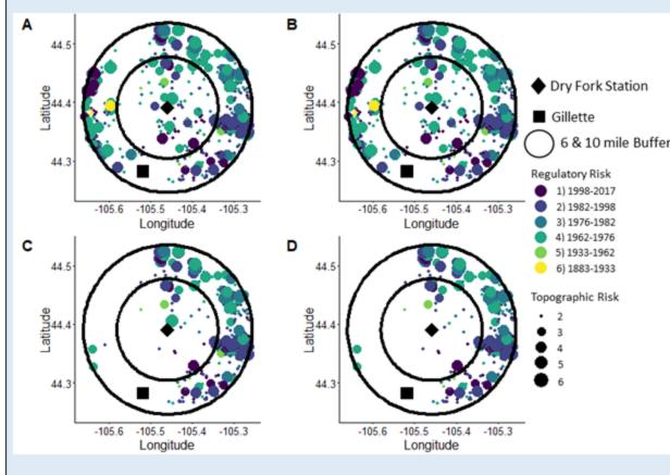
Figure 2. The risk associated with each plugged and abandoned well within ten miles of Dry Fork Station. The size of the point indicates the risk associated with topographic depressions, "6" being the riskiest. The color indicates the PA regulations of the time period, with yellow having the highest risk. (Table 1).
