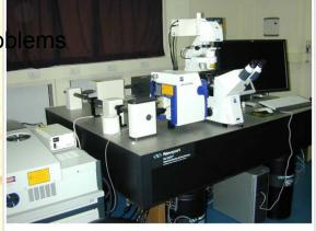
Laser scanning confocal microscope
