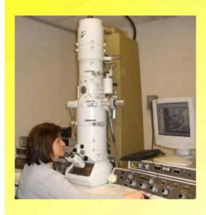
Transmission electron microscopes & similar \$1M instruments enable UW scientists to study and create nano-devices at the scale of single atoms.
