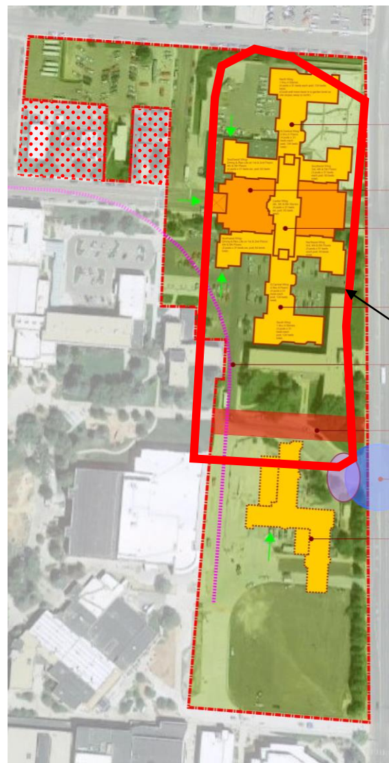
Scheme A concentrates Phase 1 program into a single large building, creating a new superblock
