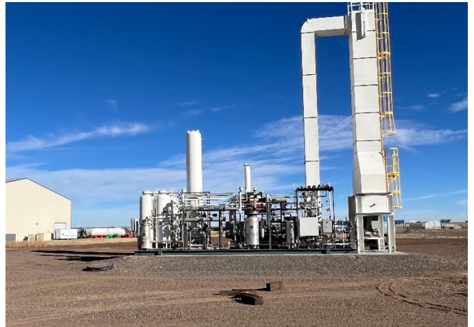
The SMR unit was fully assembled and ready for testing at the EP&C's shop in Cheyenne, Wyoming
