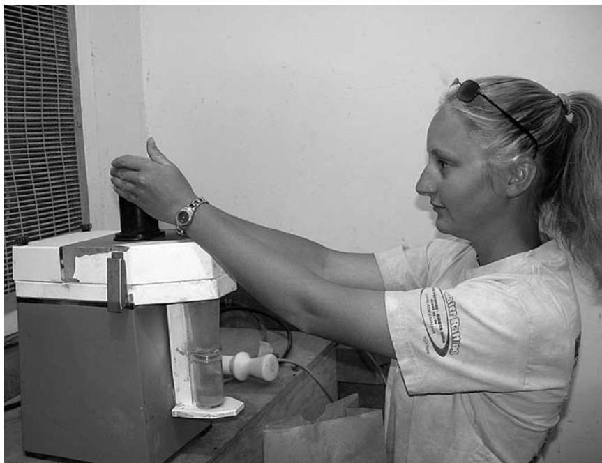
Sara Skalsky grinds samples from sugar beets to determine how much nitrogen content is left in the leaves.
