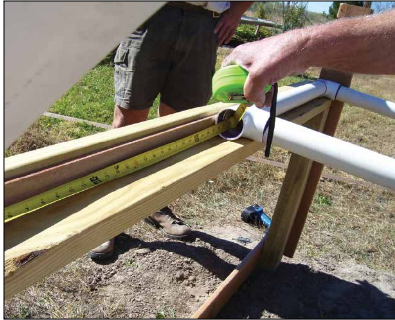
Figure 18. Measuring the distance to cut the final spacer.
