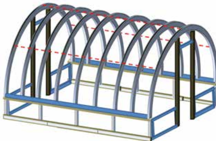
Figure 30. Red dashes indicate location of string lines for purlin locations.
