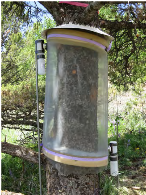
Figure 1. Completed emergence trap designed to sample natural enemies of bark beetles.
