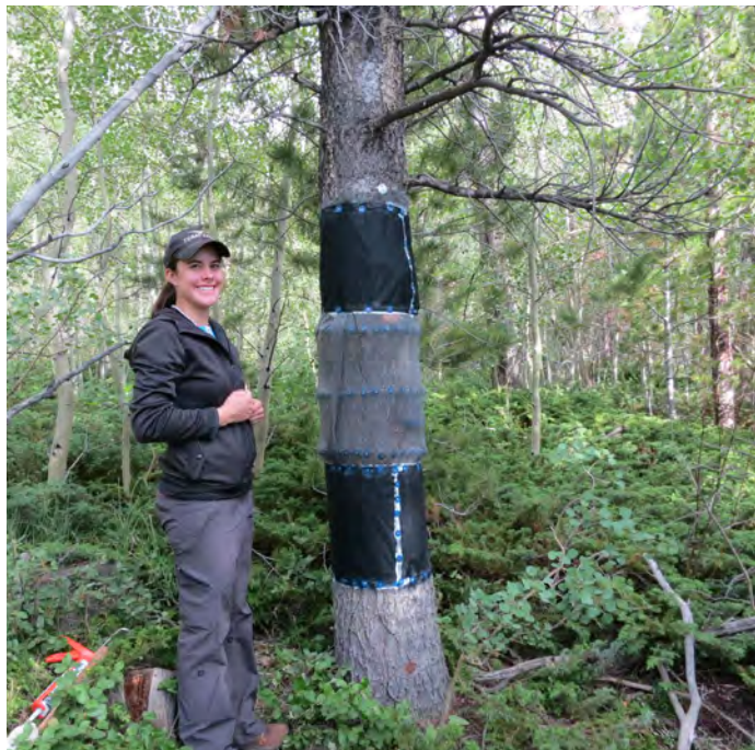
Figure 2. Research assistant Rachel Lentsch with predator exclusion cage for mountain pine beetle.
