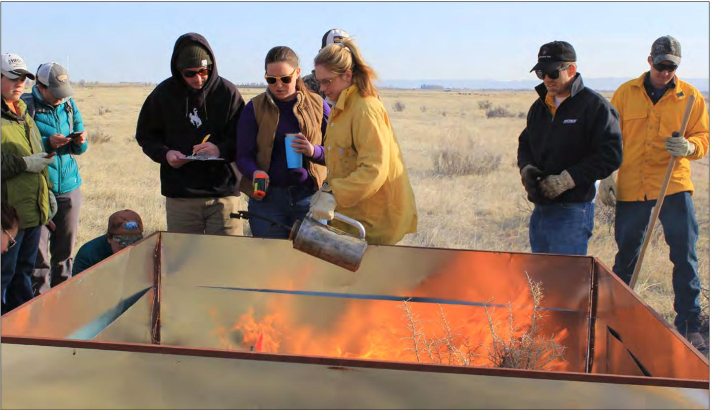
**Figure 1.** UW students started fires in burn boxes to quantify canopy and soil-surface fire temperatures in a saline-greasewood ecological site in southeast Wyoming.
