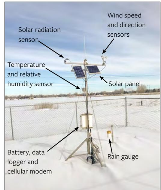
**Figure 2.** WACNet automated weather station at Worland.
