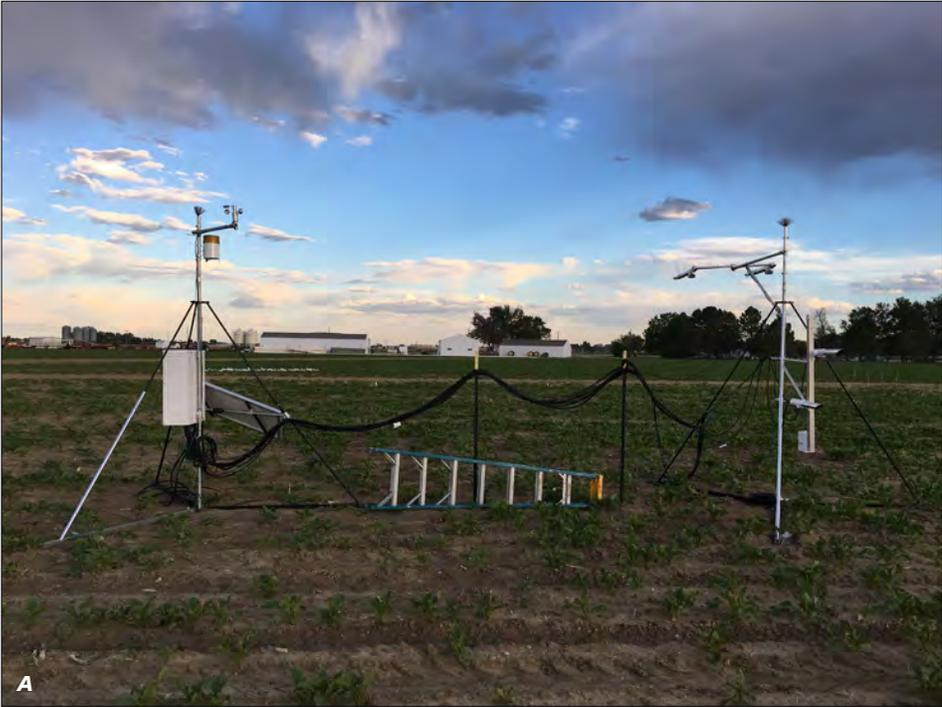
**Figure 2.** Bowen ratio-energy balance system for measuring crop evapotranspiration and crop coefficients during the growing season (A); and for measuring evaporative losses during the non-growing season (B).
