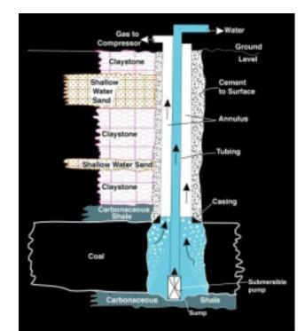
This is a typical production schematic for a coalbed methane well.
