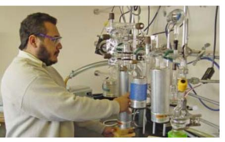
Enrico Yepez, a doctoral student from the University of Arizona who is assisting in the isotope lab, loads a sample of ground grass into a tin capsule to be heated. It will react with oxygen to form carbon dioxide from the organic material sample that will be analyzed in a mass spectrometer.
