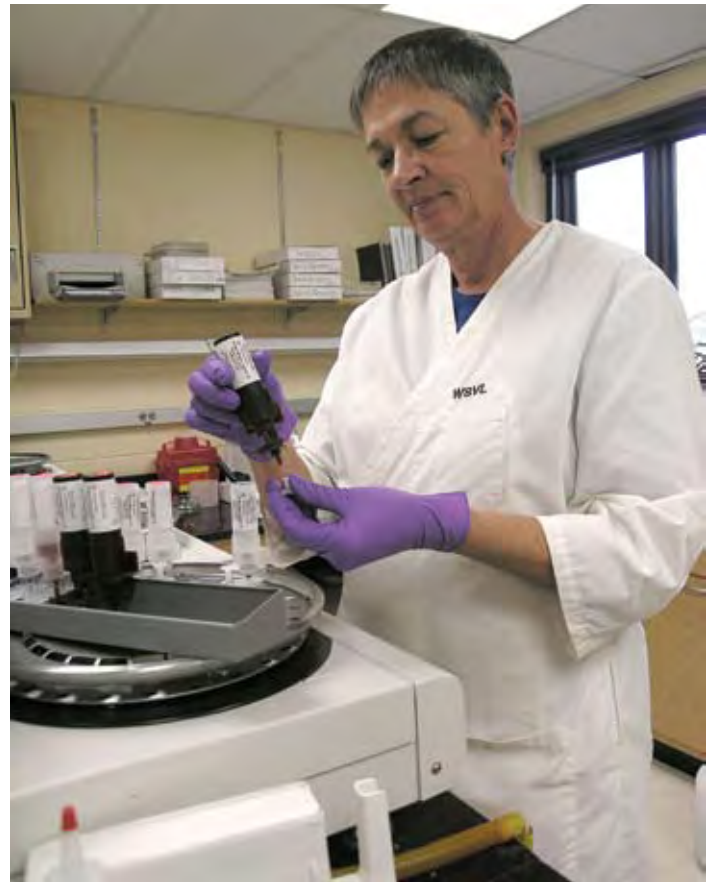
Certified histotechnologist and lab supervisor Paula Jaeger prepares the automated instrument for chronic wasting disease immunohistochemical staining. This instrument can stain 80 slides per run.
