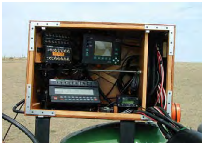
The controls on a precision crop sprayer, including the rate controller, field computer, boom controls, and Global Positioning System receiver.
