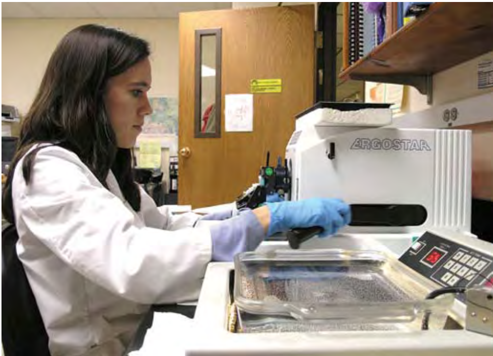
Using a rotary microtome, certified histotechnologist Mercedes Thelen prepares tissue sections for chronic wasting disease (CWD) staining. In 2005, the pathology laboratory prepared 10,037 CWD slides for the pathologists to examine.
