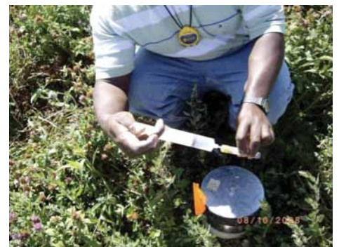
Collection of gas samples for analysis of greenhouse gas emissions (carbon dioxide, nitrogen dioxide, and methane) in different sugar beet cropping systems in the Big Horn Basin.
