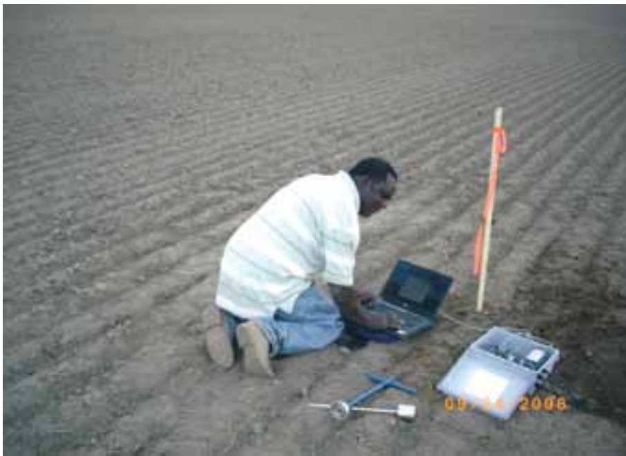
Eusebius Mukhwana, a Ph.D. student in soil science, downloads data from automated moisture and temperature sensors installed in different cropping systems. The system collects moisture and temperature information at five soil depths every 30 minutes.
