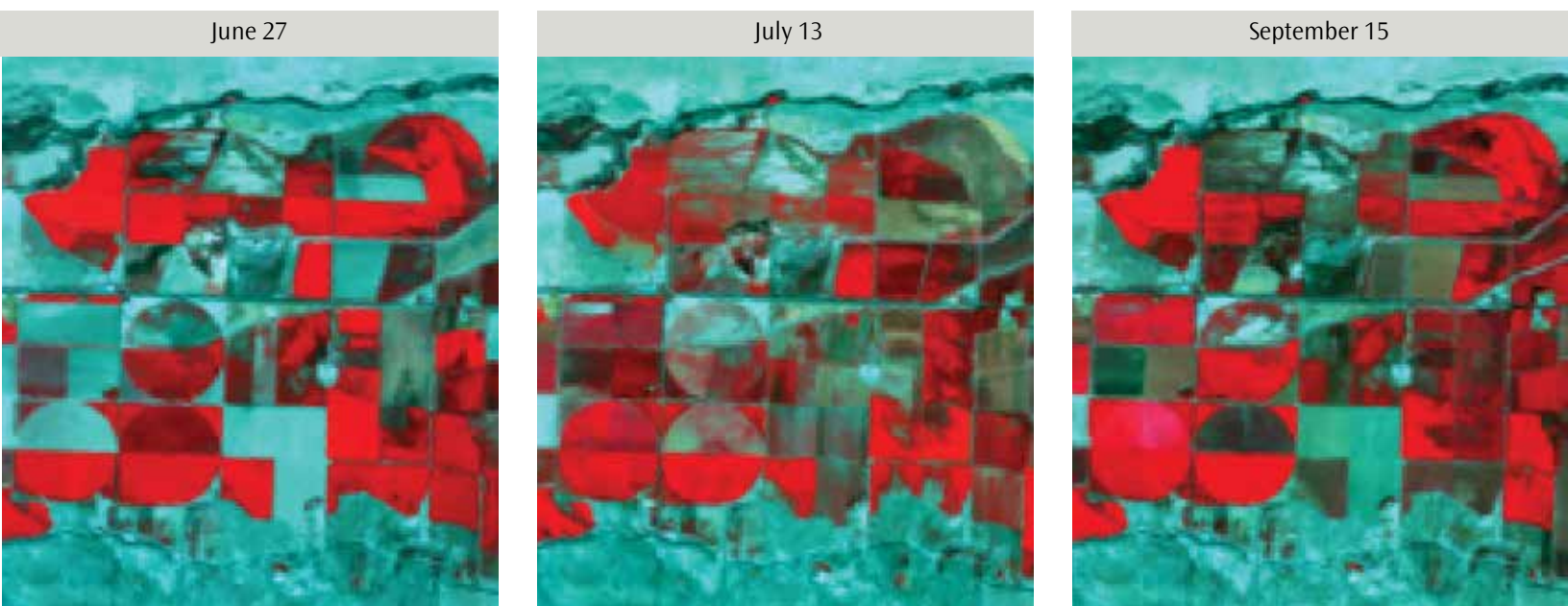
Infrared images acquired by a Landsat satellite show changes in crop growth during the 2007 growing season. Crops with high growth (or vigor) appear bright red due to more reflection in the infrared region. Darker shades of red indicate medium- to low-growth areas. Harvested areas and bare ground appear in shades of green and blue.
