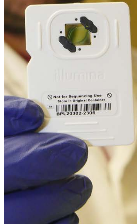
Brian Dominguez of the WSVL's sequencing and bioinformatics unit holds a reusable flow cell used to perform maintenance on DNA sequencing equipment. Photo by David Keto.
