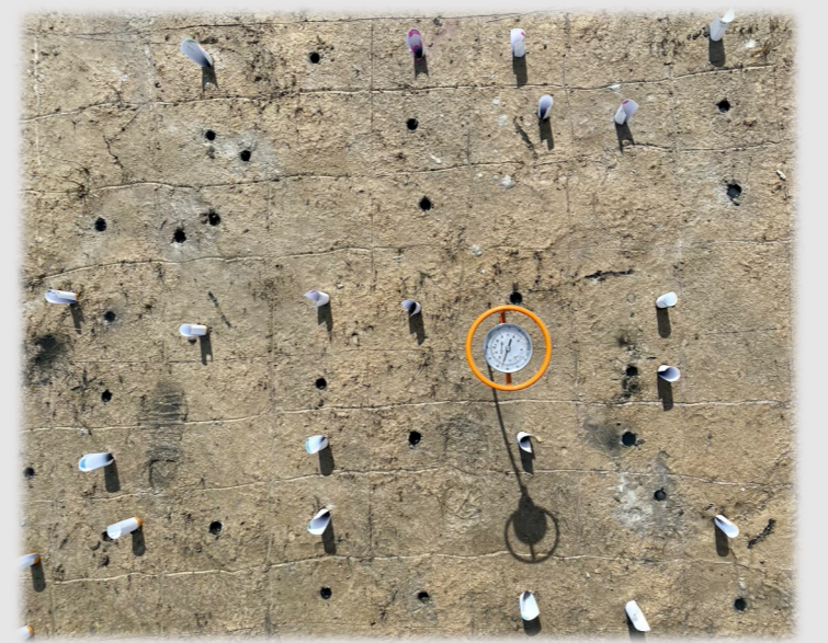
Figure 2. IRIS films were randomly installed in a grid. Soil temperature was measured at 25 cm throughout the study.
