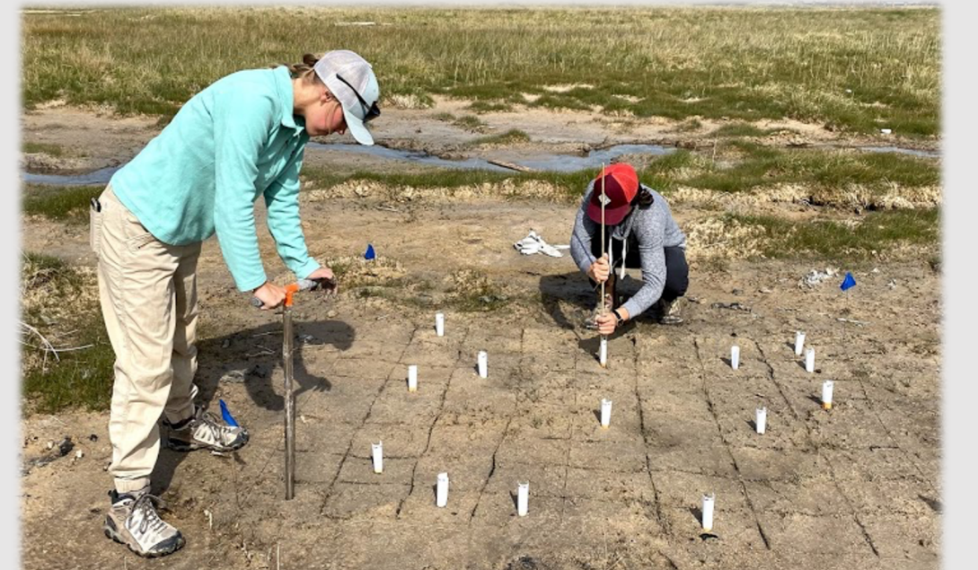
Figure 5. Soil is extracted using the probe while the IRIS films are deployed.
