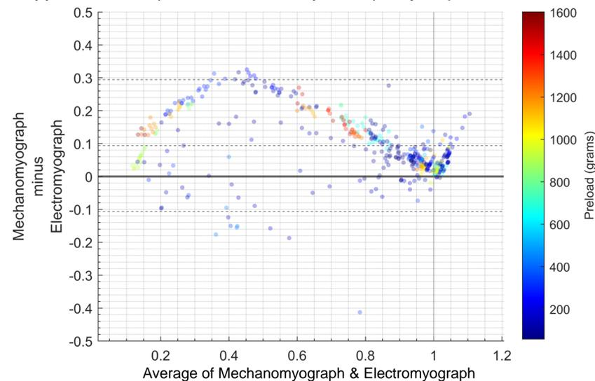
**Figure 3.** Bland-Altman plot comparing clinical electromyograph readings to mechanomyography device measurements. Data points are color-coded to represent thumb preload at various train-of-four ratios. 491 train-of-four ratio data points were collected for paralyzed patients.
