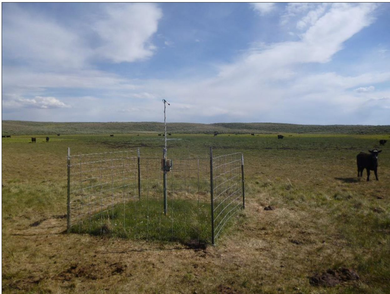
Figure 2. ARU deployment with fenced enclosure, SongMeter2 recording unit, and ultrasonic microphone.
