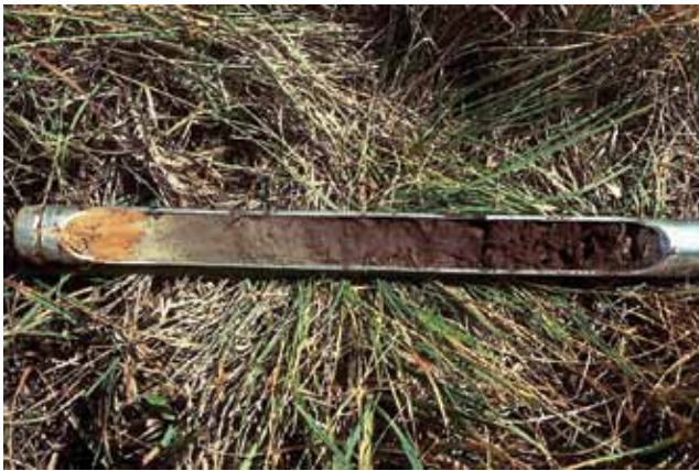
Figure 10 —A soil core collected from a mound showed evidence of oxidized iron in the mineral portion at the base (left side of photo), indicating fluctuating water table and seasonal aerobic conditions (photo: Bonnie Heidel, WYNDD).
