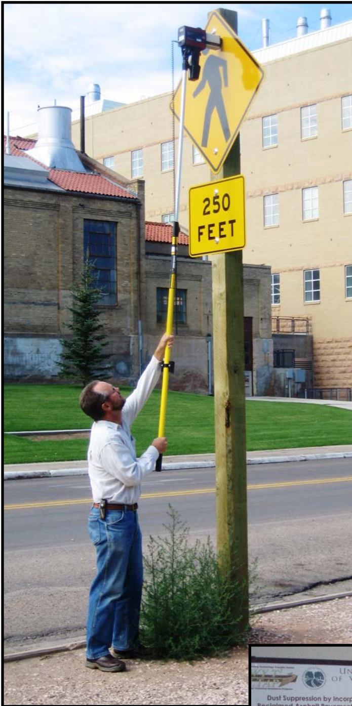
Above: George checking retroreflectivity on a pedestrian crossing sign on the UW campus. Right: George presenting information on Dust Suppression by Incorporating Reclaimed Asphalt Pavement into Gravel Roads
