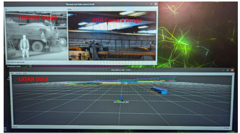
Figure 4: Display inside the Snowplow cabin for multiple sensor/camera-based vehicle detection.
