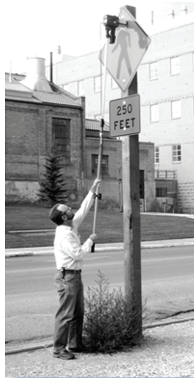
George Huntington demonstrates the use of the retroreflectometer using the extension for taller signs.
