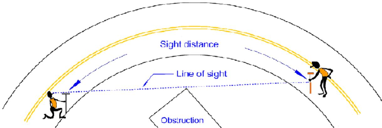
Use the Table in Figure 25 to determine if the stopping sight distance is acceptable for the speed limit and traffic volumes.
