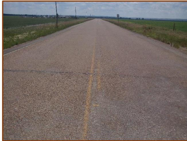
Figure 9 presents a roadway that may receive a score of three in the ROW/Shoulder category for the absence of an adequate shoulder. It may also receive a score of five in the Signage and Pavement Marking category because of the poor visibility of an advisory speed limit and reduced speed ahead sign. It also has a faded centerline. However, it may be given a score of nine in the other three categories due to the satisfactory conditions in terms of these categories.
