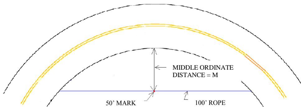
Use Figure 22 to find the radius and degree of curvature of the curve that corresponds to the measured middle ordinate.
