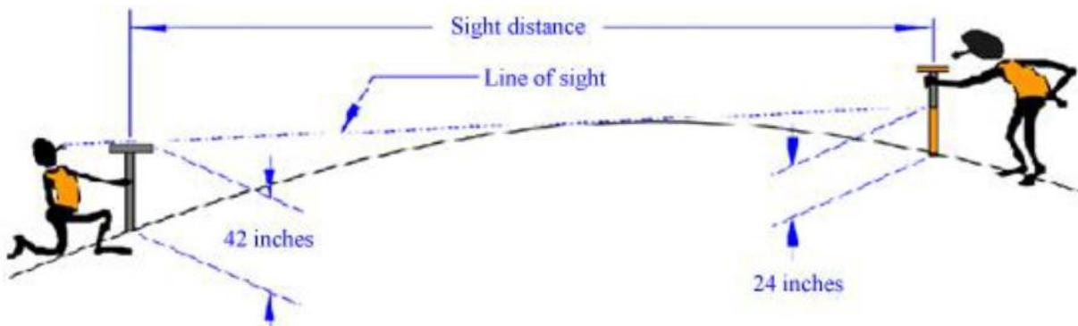
Use the stopping sight distance in Figure 25 to determine if the measured stopping sight distance is acceptable given the speed limit and traffic volumes.
