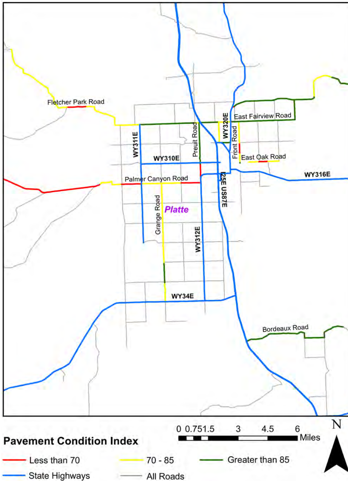
Appendix 7.16.3: Pavement Condition Index (PCI) in Platte County.
