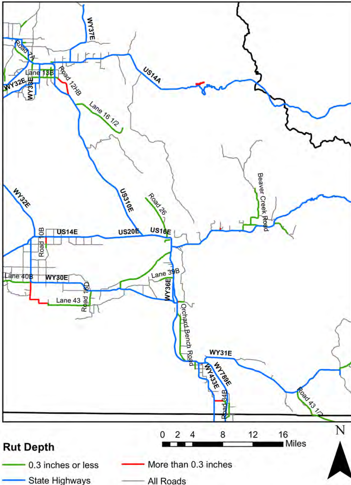
Appendix 5.2.3: Rut Depth Conditions in Big Horn County.
