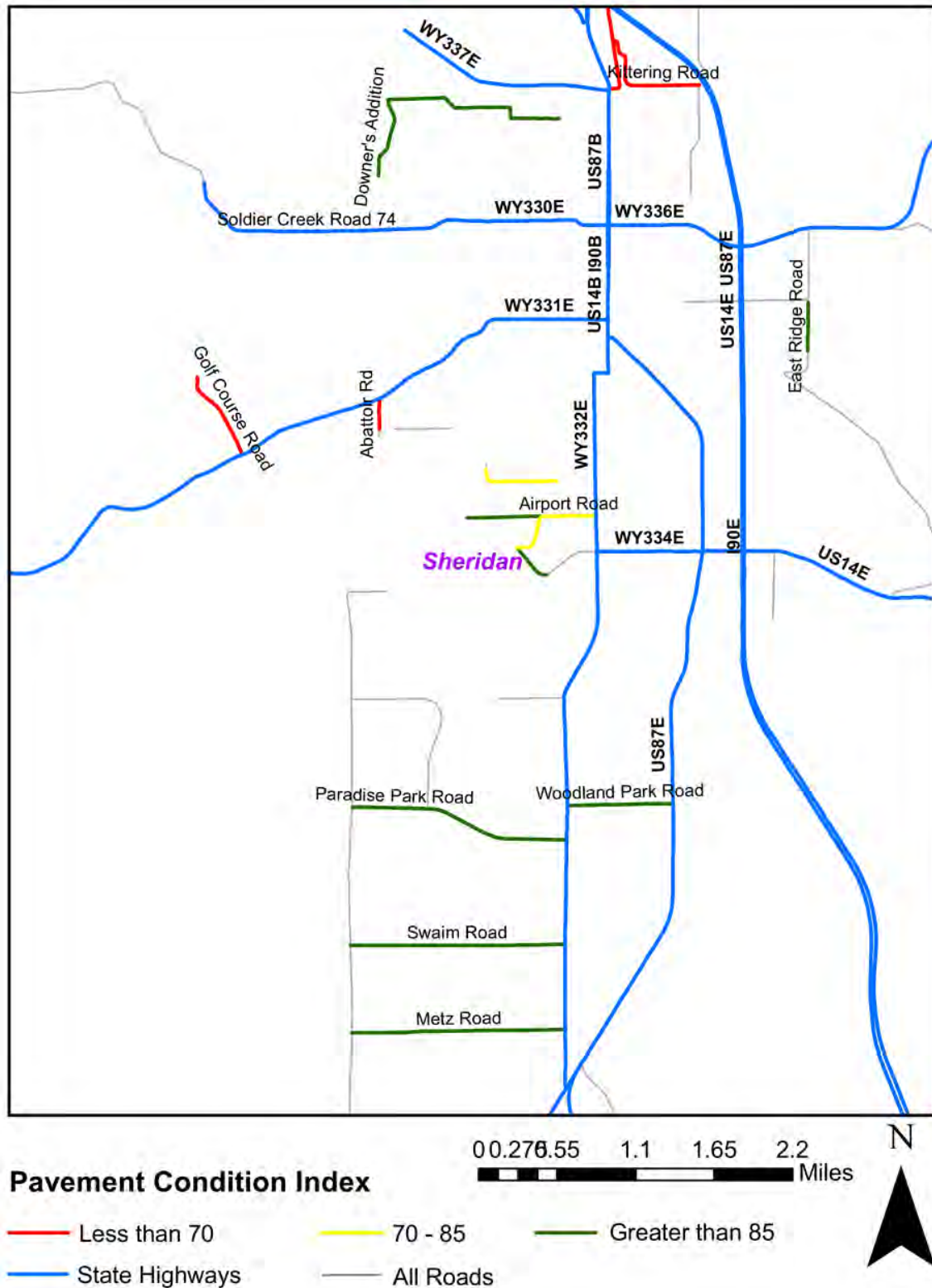
Appendix 7.17.3: Pavement Condition Index (PCI) in Sheridan County.
