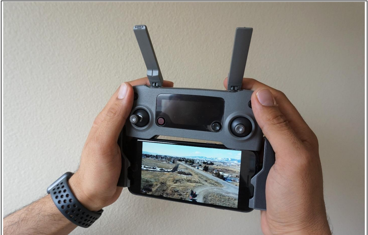
Figure 9: Many prosumer UAS rely on a smartphone or tablet device to act as a view monitor and to provide computing capacity to operate third-party applications to control the UAV, collect/record data and to plan flight activities by checking airspace and weather conditions.
