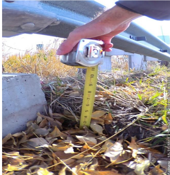
Figure 10. The elevation of accumulated dirt at the bottom of posts in site No. 2.
