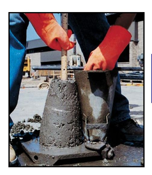
Amount of water to produce a given slump increases with increasing concrete temperature
