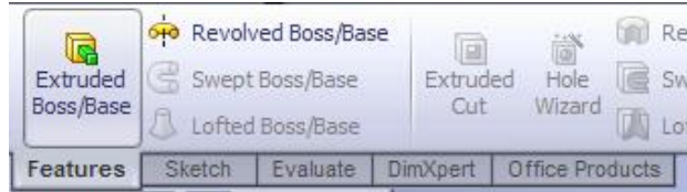
Figure 7. Extruded Boss/Base tool in the Features tool bar.
