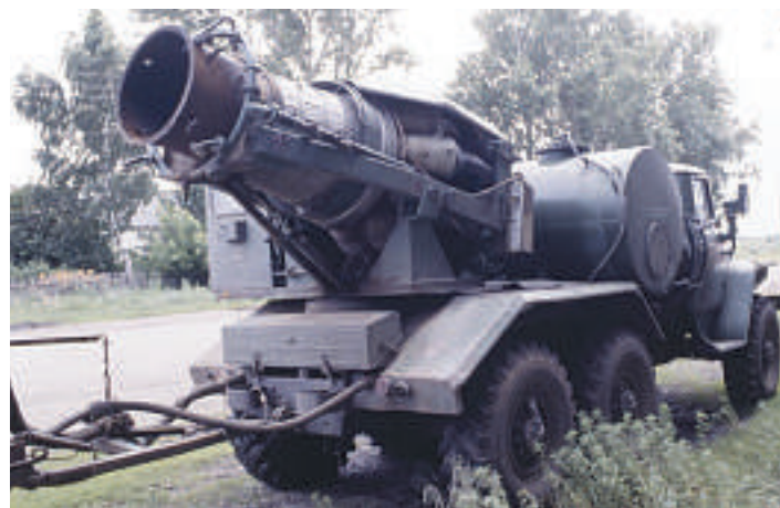
Figure 6. Giant aerosol fogger based on jet engine used in locust control in Kazakhstan (photo by A. Latchininsky).
