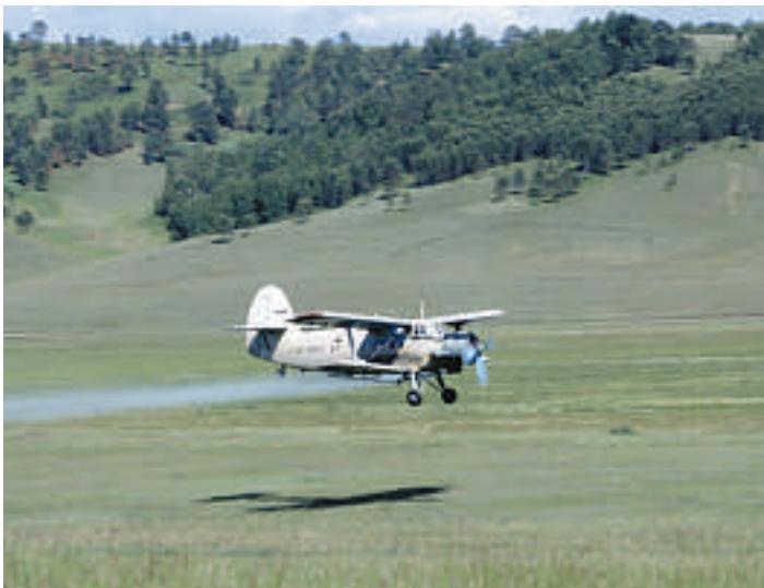
Figure 2. Anti-grasshopper insecticide spraying from ANTONOV-2 aircraft in Siberia (photo by A. Latchininsky).
