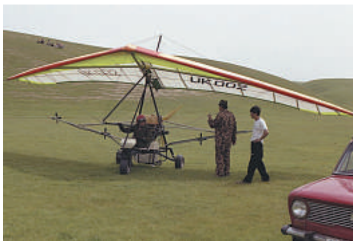
Figure 7. Ultra-light aircraft with ULV spraying equipment for locust control in Uzbekistan (photo by A. Latchininsky).
