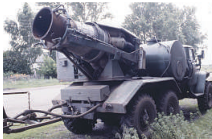
Figure 6. Giant aerosol fogger based on jet engine used in locust control in Kazakhstan (photo by A. Latchininsky).
