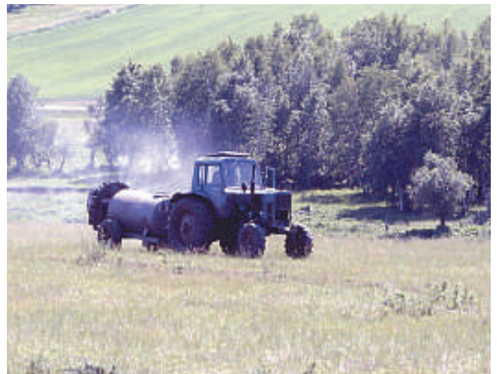
Figure 4. Tractor-driven ventilator sprayer at work against grasshoppers in Siberia (photo by A. Latchininsky).
