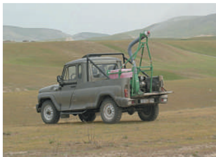
Figure 8. Micron Sprayers AU8115 atomizer mounted on Russian UAZ light truck spraying the Moroccan locusts in Uzbekistan (photo by S. Krull, GTZ).
