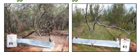
We collected runoff and sediment from six 1-x 5-m plots in FS and 4-y sites on both soil types (24 plots total). Runoff water was quantified and nutrient content measured. Sediment was quantified.
