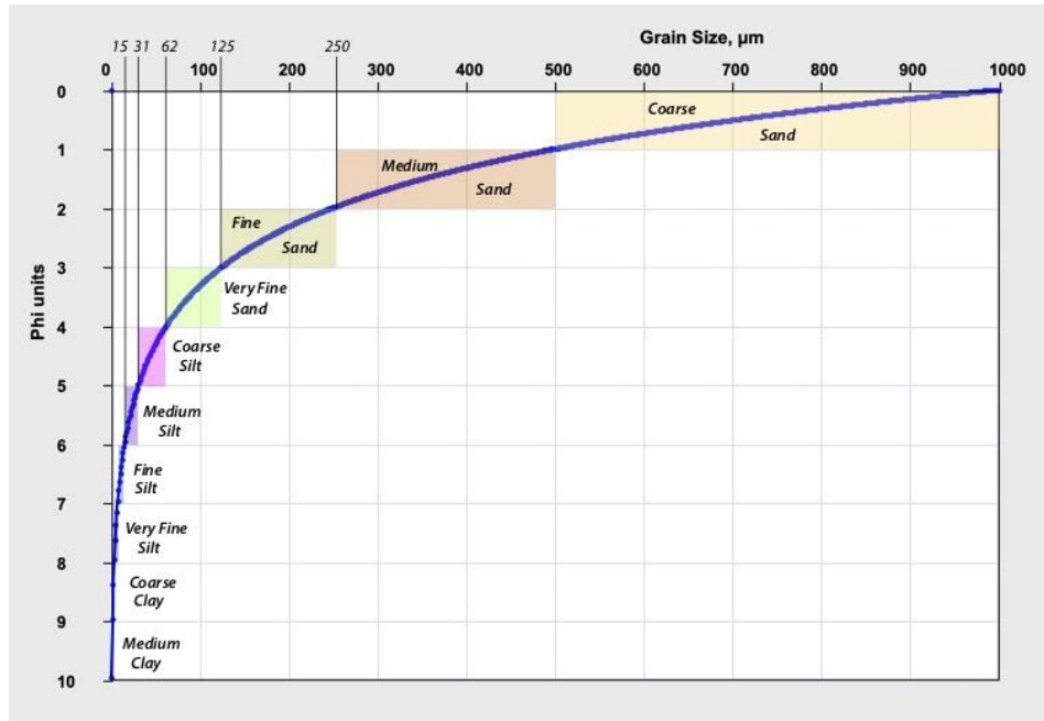
Figure 2. Interpretive grade scale chart relating rocks' grain size (in micrometers) to the logarithmic Phi scale. Based on Udden-Wentworth (1914 and 1922) and Krumbein's (1934) publications.
