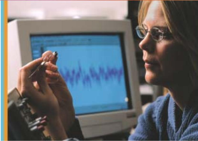
*Jenny Newton, a UW master's candidate in electrical engineering, prepares a fly for measurement of the insect's electrical response to edge images produced by a green laser.*
